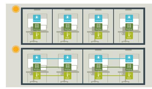
Desigo™ Total Room Automation offers maximum flexibility. With its advanced segment concept, the building floor plan and the room layout can be adjusted easily and quickly – without modifying electrical or HVAC installations.
