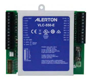
The Alerton® VisualLogic® VLC-550-E is a versatile, BACnet-compliant, fully programmable field controller designed for fan coils, a/c-units, heat pumps, and other terminal unit applications. As a native BACnet controller, it integrates seamlessly with your BACnet system, communicating at up to 115 Kbps on a BACnet MS/TP LAN.
