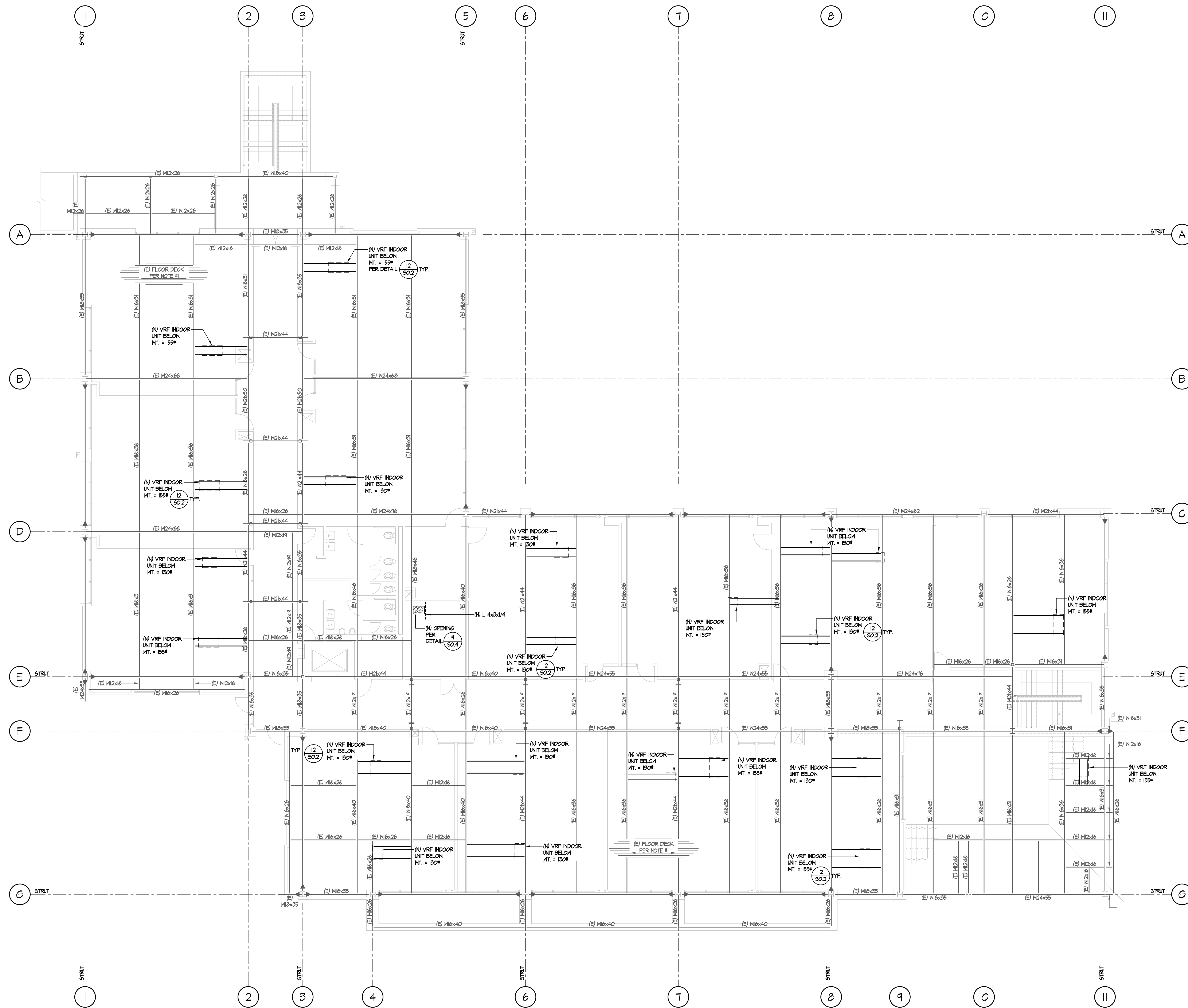
BLDG. 'C' SECOND FLOOR FRAMING PLAN SCALE: 1/8"=1'-0"
