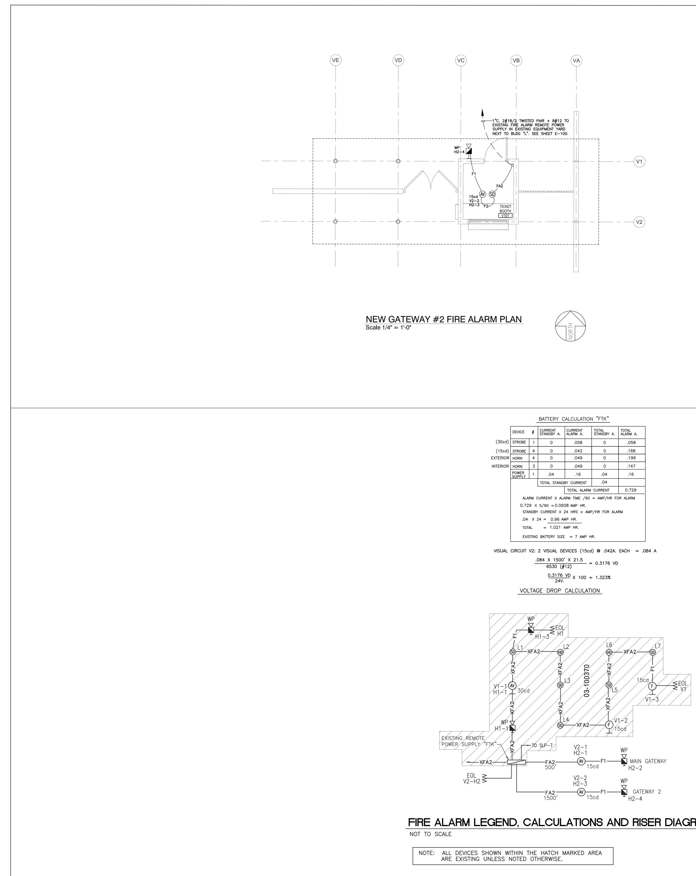
FIRE ALARM LEGEND, CALCULATIONS AND RISER DIAGRAM
