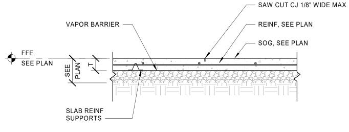
E3 SLAB ON GRADE CONTRACTION JOINT DETAIL S2.1 3/4" = 1'-0" <u>NOTES</u>: 1. CUT EVERY OTHER REINF WHERE CONTRACTION JOINTS ARE TO BE CUT. SAW CUT SLAB WITHIN 8 HOURS OF CONCRETE POUR.
