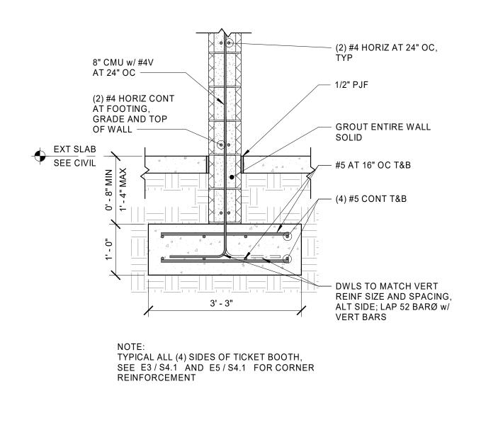
A3 SECTION AT EXTERIOR TICKET BOOTH MASONRY WALL S4.1 3/4" = 1'-0"
