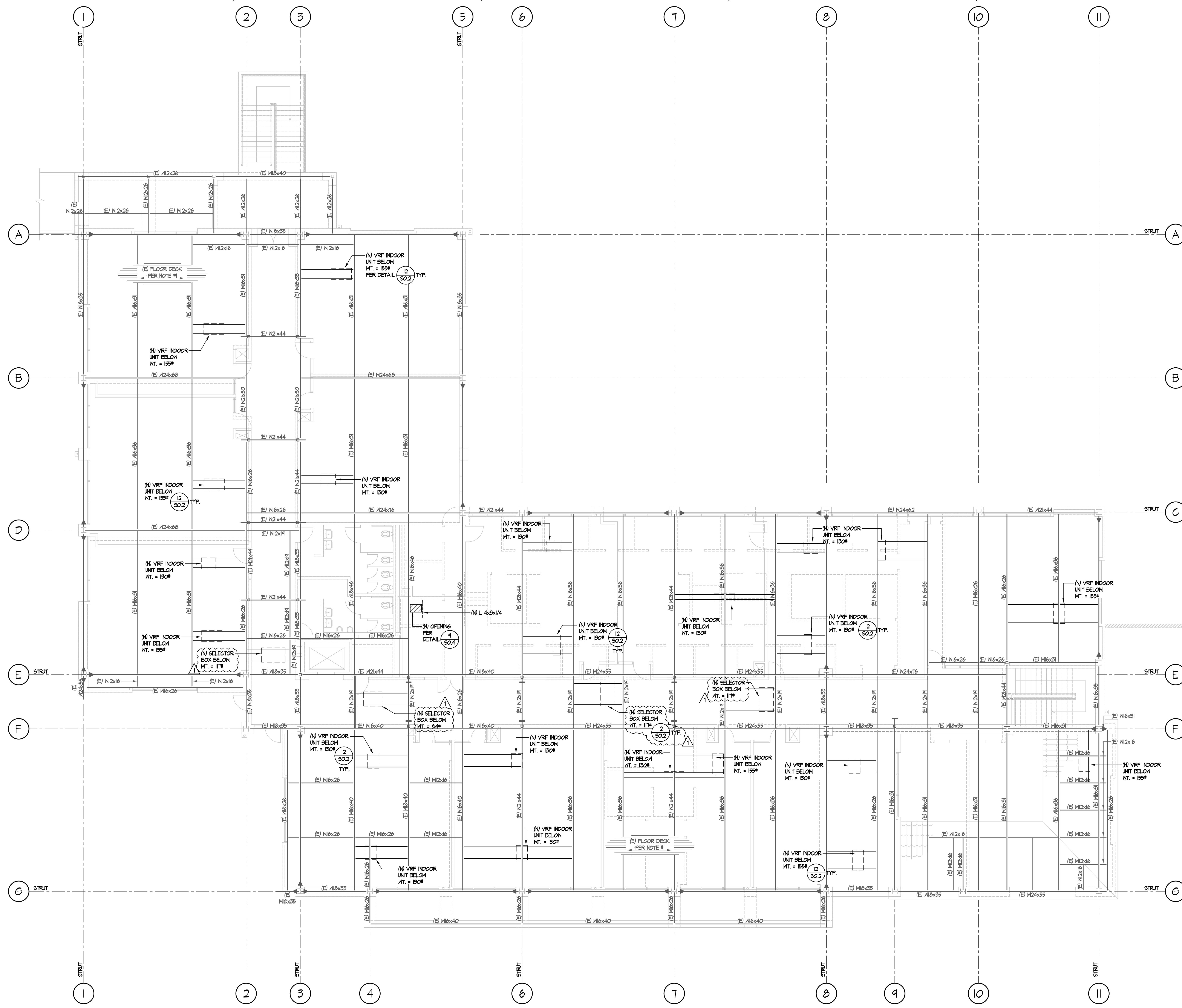
BLDG. 'C' SECOND FLOOR FRAMING PLAN SCALE: 1/8"=1'-0"
