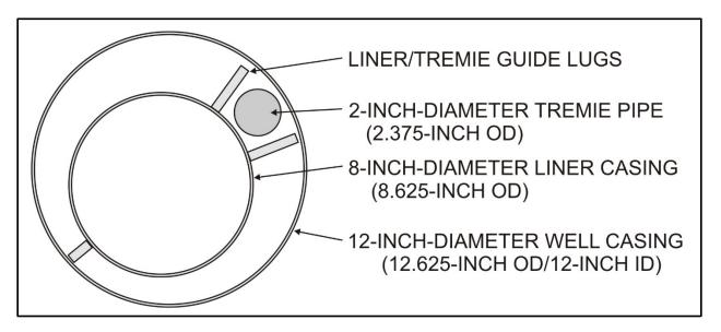
Figure 3 - Tremie and Liner Guide Lug Placement
